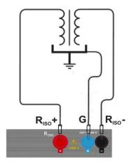
when measuring insulation resistance between one of the cable conductors and the cable jacket, the effect of surface resistances (important in difficult weather conditions) is eliminated by connecting a piece of metal foil insulating the tested conductor with G socket of the meter;
