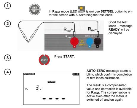
In order to remove the compensation of the leads resistance (return to default calibration), perform the above-mentioned activities with test leads open, instead of test results, the display will show message **oFF** (compensation of test leads is turned off).
