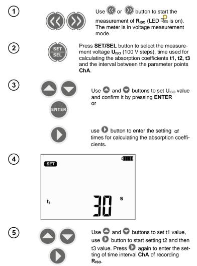
Defining ChA interval will enable the user, using Sonel Reader software, to plot the resistance chart and current chart using the data obtained from the performed measurement (see example below).
