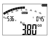
After the measurement is completed or stopped, read the result. The results of all completed measurements will be displayed (even when the measurement was interrupted/stopped e.g. after 60 seconds). When the meter switched into standby mode, the measurement result may be recalled by pressing ENTER.
