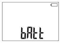
The battery pack is fully discharged, all measurements are blocked. The meter switches off automatically after 5 sec.
